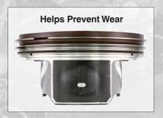
After 1,000 miles (1,609 km) of extreme-heat dyno testing, AMSOIL 20W-50 Synthetic V-Twin Motorcycle Oil protected against piston-ring sticking and piston scuffing for maximum compression and power.
